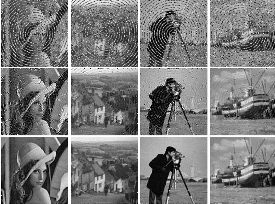
Figure 3: The restored results of images blurred by fspecial('disk', 3) and corrupted by random-valued noise (level s = 36.83\% ) at specific set and Gaussian noise (STD \sigma = 5 ). Top row: blurry and noisy images; Middle row: the results restored by Fast_IFASDA; Bottom row: the results restored Ada_Fast_IFASDA.
