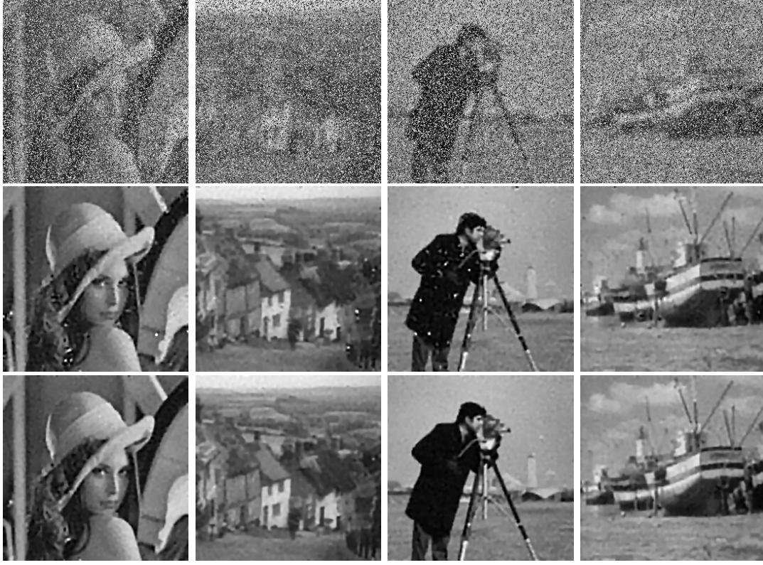
Figure 2: The restored results of images blurred by fspecial('disk', 3) and corrupted by random-valued noise (level s = 55\% ) at random set and Gaussian noise (STD \sigma = 5 ). Top row: blurry and noisy images; Middle row: the results restored by Fast_IFASDA; Bottom row: the results restored Ada.Fast_IFASDA.
